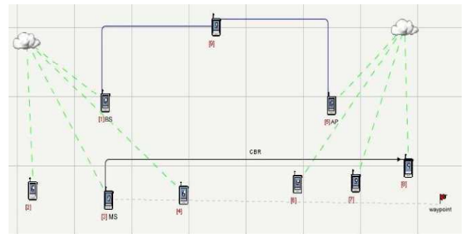
Figure 5. The QualNet simulation scenario of WiMAX and WiFi networks
